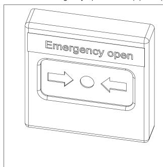
In the event of a system failure or panic, the emergency escape switch can be operated to bring the system into the safety position.
