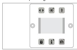
The BDE-D operating unit is an input and output unit for the operation and limited programming of the system. The display shows information about the system by means of symbols and text.
